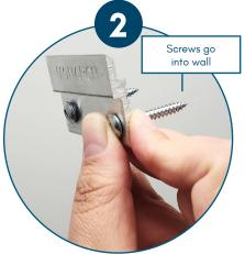
You will be provided the appropriate amount of Monarch Z Clip(s) along with 2 screws per clip. The ridged part of product faces the back (wall). The Screw holes face the bottom. The lip should be facing up. (Sometimes the Monarch writing will appear upside down).
