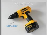
If the wall is hard plaster and you can't push-in the peg, you need to drill pilot holes.
