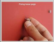
If a peg ever gets loose, fill the hole with a bit of wood and re-insert the peg.
